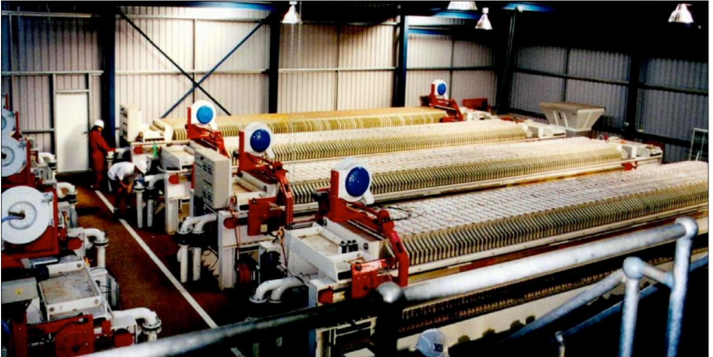
Pressing section with Filer-Presses FP 12-D12-M - Sydney
