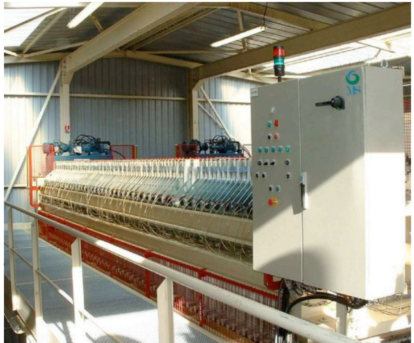
Pressing section with Filer-Presses FP 12-D12-M - Sydney
