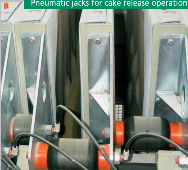
Pneumatic jacks for cake release operation
